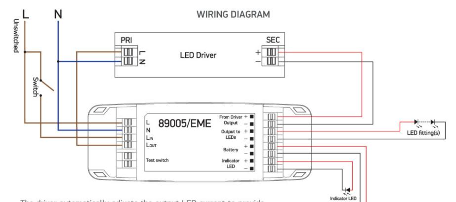
The driver automatically adjusts the output LED current to provide the optimum match between the battery and the load, providing maximum illumination whilst ensuring full battery duration.
