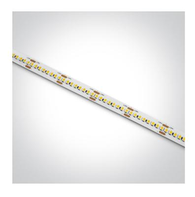
Flexible LED light strip, with SMD2835 LEDs, 240LEDs/meter, 42W/meter.Supplied in 2 meters roll with white PCB and double adhesive tape for a better fixing.
