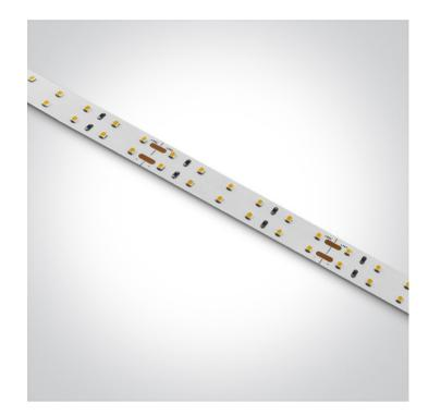
Flexible LED light strip, with SMD2835 LEDs, 120LEDs/meter, 28,8W/meter.Supplied in 5 meters roll with white PCB and double adhesive tape for a better fixing.
