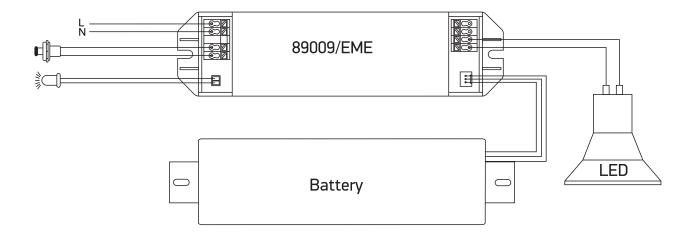
$^{\ast}$  This kit will only operate with GU10 / E27 LED lamps suitable for 180V DC power supply.
