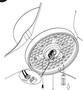
Install LED plate and connect cable.
