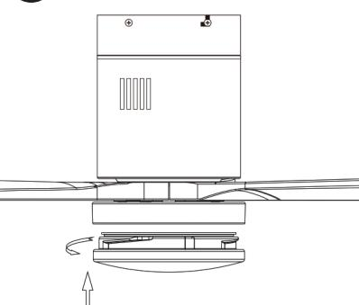
Install the diffuser onto the LED plate.
