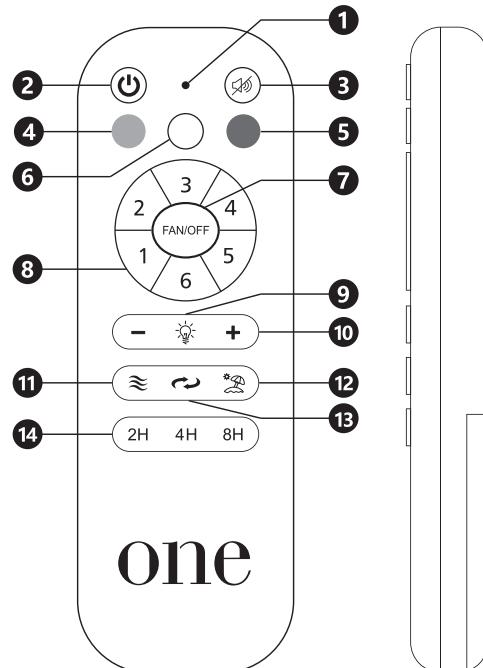
NOTE: To pair a remote to a receiver turn ON the power supply to the fan and press the ON/OFF and MUTE keys on the remote for 3 to 5 seconds. You will hear a beep.
