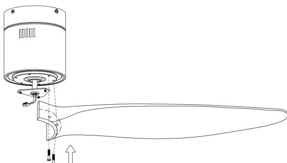
Install the fan blades and tighten screws.
