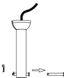
Remove the R clip from the pin. Then remove the pin from the rod.
