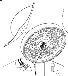
Install LED plate and connect cable.
