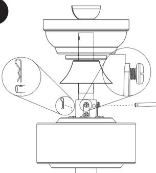
**A** Put the rod into the motor and install the pin and R clip.
