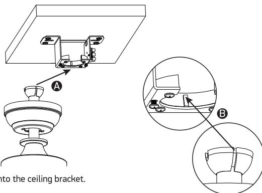
**A** Hang the fan onto the ceiling bracket.
