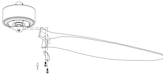
Install the fan blades and tighten screws.
