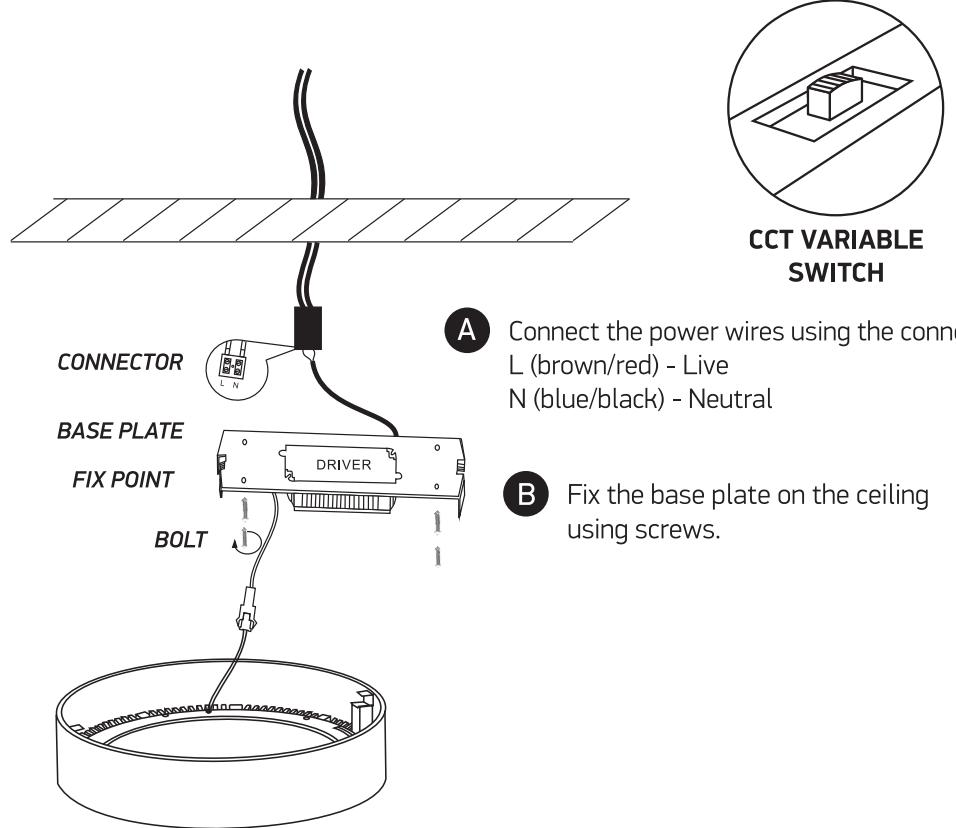
**A** Connect the power wires using the connector.
