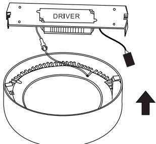
D Close the fitting by turning it clockwise,
