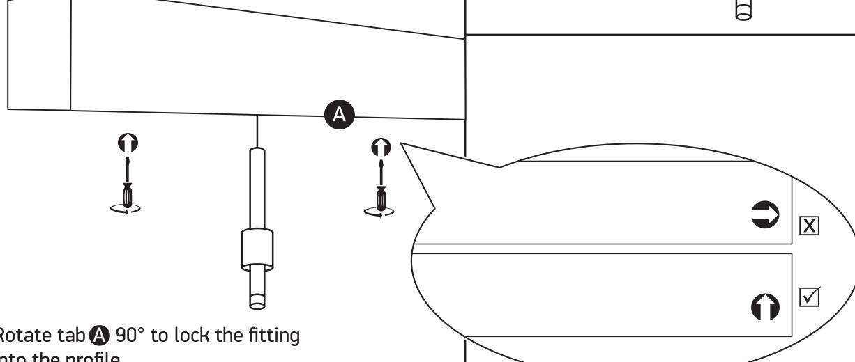
Rotate tab A 90° to lock the fitting into the profile.
