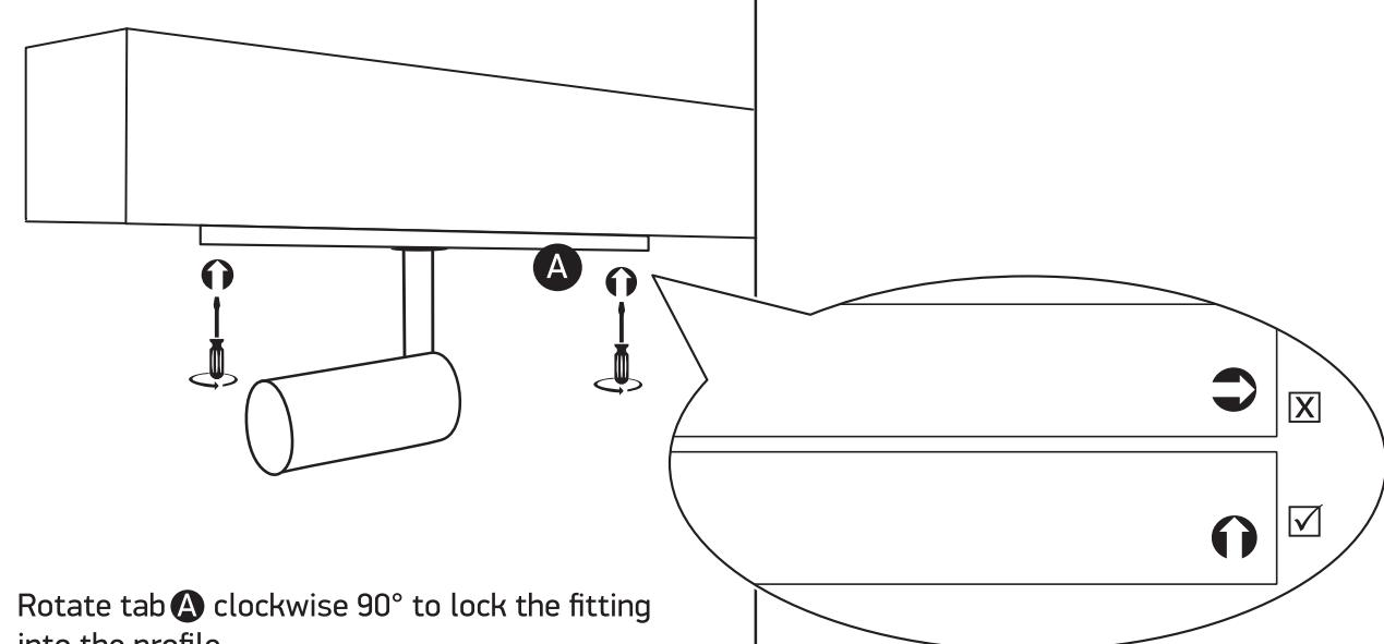
Rotate tab A clockwise 90° to lock the fitting into the profile.
