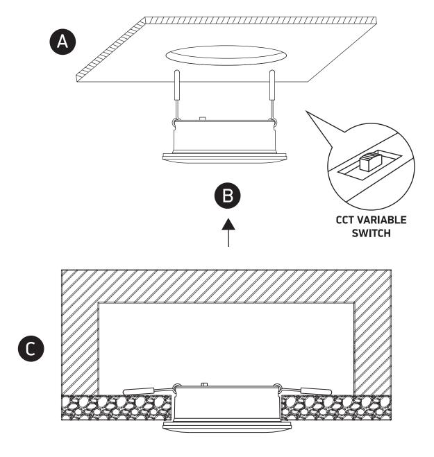
\*IP65 is the protection degree for the visible part of the fitting under the ceiling. The part of the fitting hidden in the ceiling is IP20.
